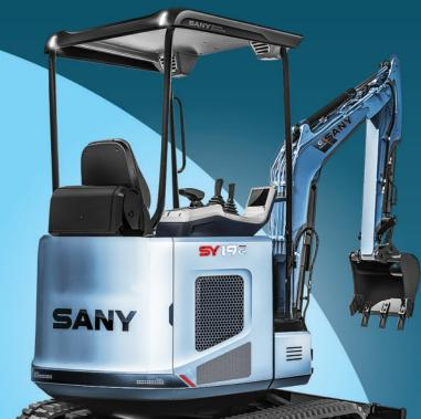
As well as zero emissions and considerably lower noise levels, the compact electric SY19E is equipped with a lithium iron phosphate (cobalt free) battery which allows for faster, safer and more efficient charging as well as a significantly longer battery life to reduce total cost of ownership.
